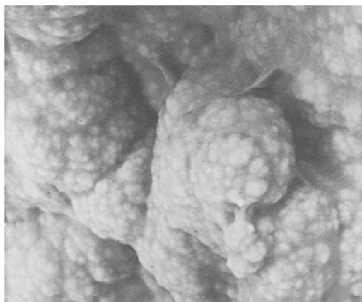
Fig. 1. Scanning electron micrograph of polypyrrole film grown at 25°C in propylene carbonate/tetra-ethyl ammonium p -toluene sulphonate system. \times 43 .
